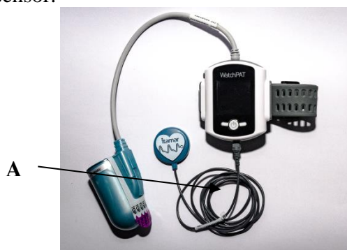
A - Integrated RESBP sensor
