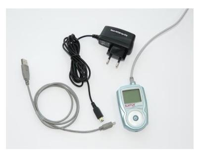
Figure 6 – Charging the WatchPAT™ device
