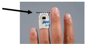
Figure 32 - Flexiwrap Line Indication
