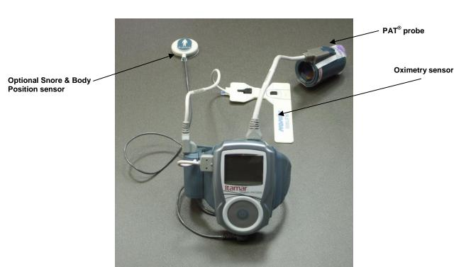
Figure 1 - Packed Device
