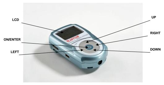
Figure 3 - The Buttons and Display
