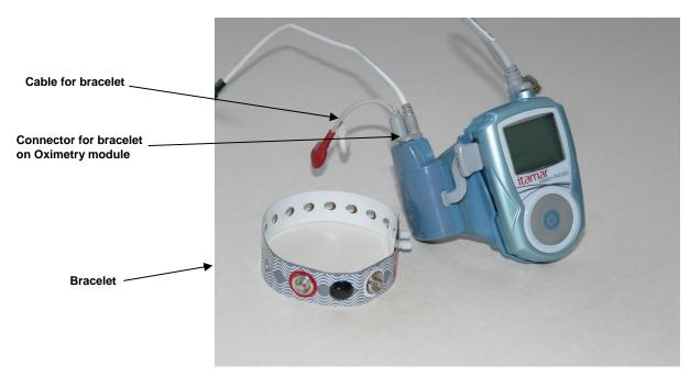
Figure 14 - WatchPAT™ Device with Tamper-Proof Bracelet
