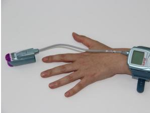
Figure 22 - Wearing the WatchPAT™ Device
