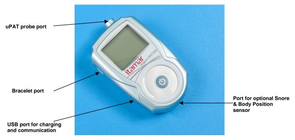
Figure 4 - Service Ports and Peripherals
