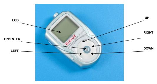
Figure 3 - The Buttons and Display
