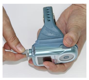
Figure 18 - Replacing the uPAT Probe
