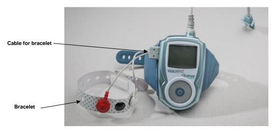
Figure 10 - WatchPAT™ Device with Tamper-Proof Bracelet
