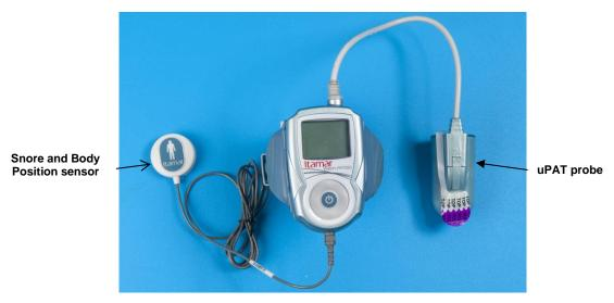
Figure 9 – WatchPAT™ Fully Prepared
