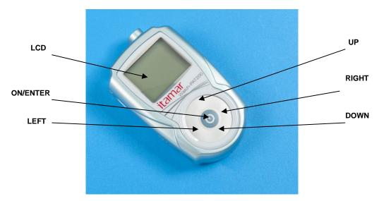
Figure 3 - The Buttons and Display
