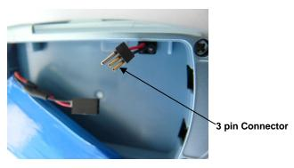
Figure 19 - Replacing the Battery
