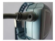
Figure 17 - uPAT Probe Cable with Screw
