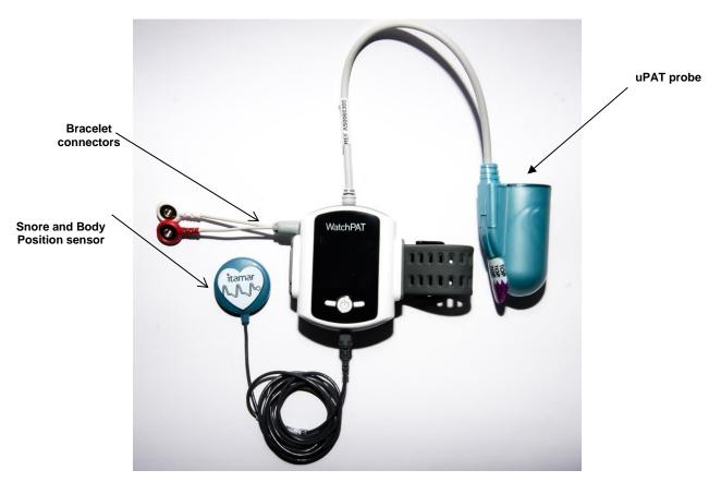
Figure 8 - WatchPAT™ Fully Prepared
