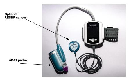
Figure 2 – WatchPAT™300 Device with Sensors
