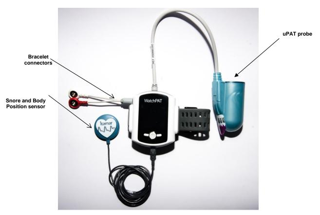
Figure 8 – WatchPAT™ Fully Prepared
