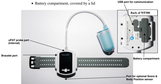
Figure 4 - Service Ports and Peripherals
