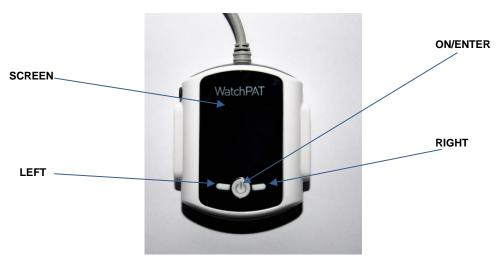
Figure 3 - The Buttons and Display
