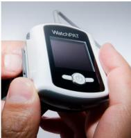
Figure 20 – Seating device on wrist strap
