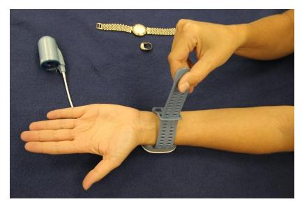
Figure 6 - Strapping the main device
