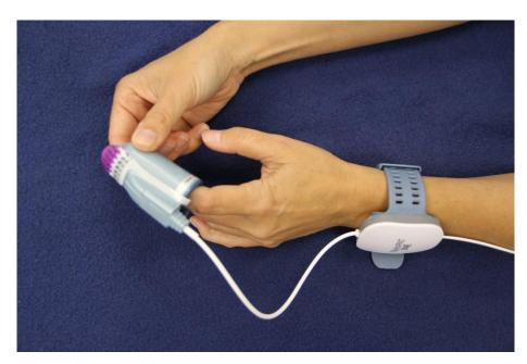
Figure 8 - Placing Finger in the Finger Probe
