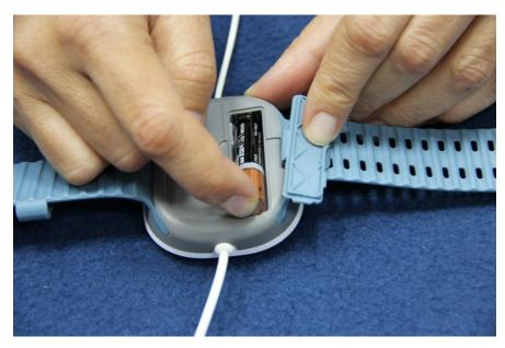
Figure 5 - Battery insertion
