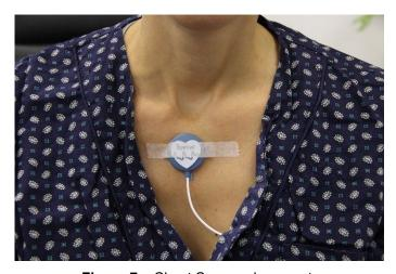
Figure 7 - Chest Sensor placement
