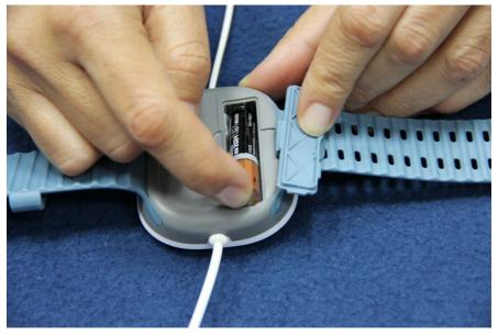
Figure 4 – Battery insertion
