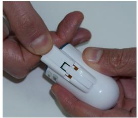
Figure 23 – New Finger probe connection
