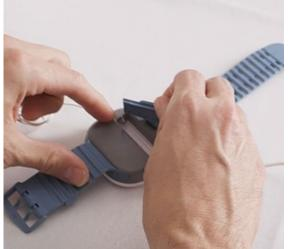
Figure 26 – **Battery removal**
