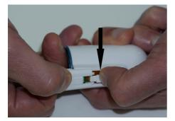
**Figure 22 – Finger probe disconnection** 1. Remove the used probe by pressing the small tab (clip) marked by the arrow, and then, holding the connector's slider, gently slide it away from the probe. Properly dispose of used probe.
