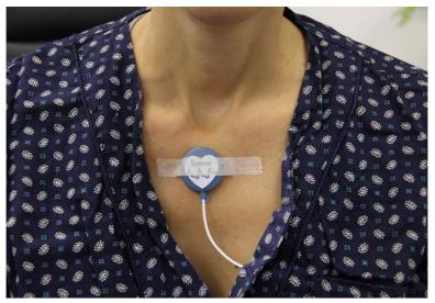
Figure 6 - Chest Sensor placement
