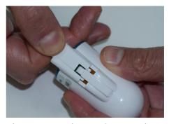
**Figure 23 – New Finger probe connection** 2. Connect a new probe by inserting the white slider to the probe until the white cover of the probe clicks into its place.
