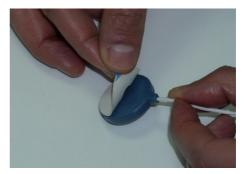
**Figure 25 – Chest sensor sticker adhesion** 4. Attach a new sticker by peeling off the cover on one side of the sticker.
