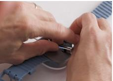
**Figure 27 – Battery insertion** 6. Insert a new disposable AAA battery. The direction of '+' and '-' is illustrated on the battery lid and inside the battery compartment.
