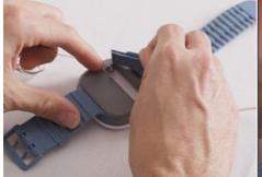
**Figure 26 – Battery removal** 5.Remove battery.
