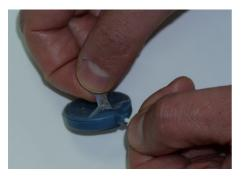
**Figure 24 – Chest sensor sticker removal** 3. Remove the used chest sensor sticker by pulling the sticker.
