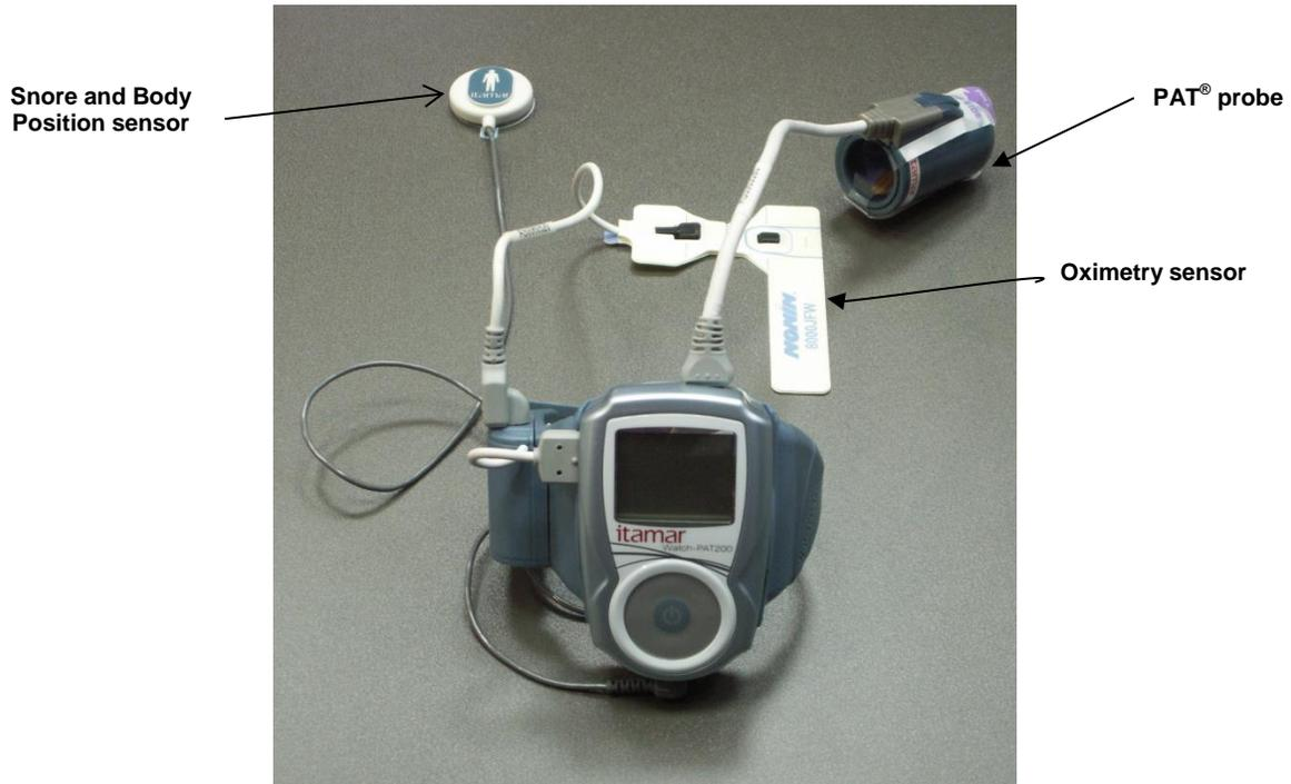
**Figure 12 – A WatchPAT™ Device Fully Prepared**
