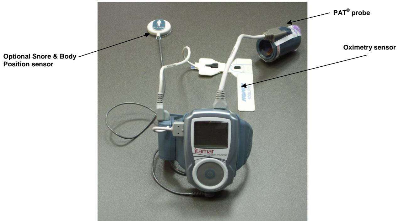
**Figure 2 – WatchPAT™ Device with Sensors**
