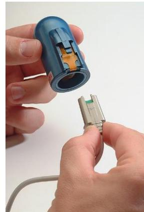
**Figure 11 – Probe Disconnected**
