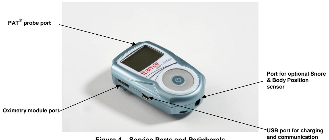
**Figure 4 – Service Ports and Peripherals**
