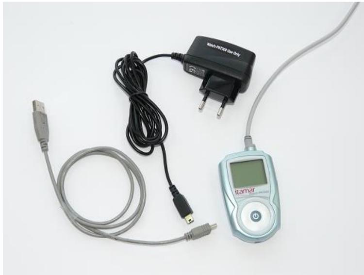
Figure 6 – Charging the WatchPAT™ device
