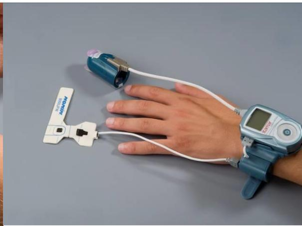
**Figure 27 – Wearing the WatchPAT™ Device**
