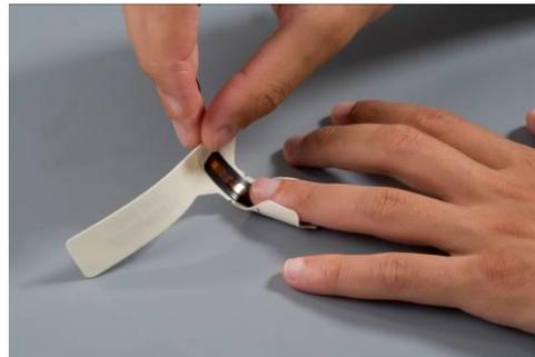
**Figure 29 – Positioning Oximetry On Ring Finger**
