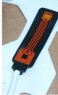
**Figure 7 – Oximetry Sensor**
