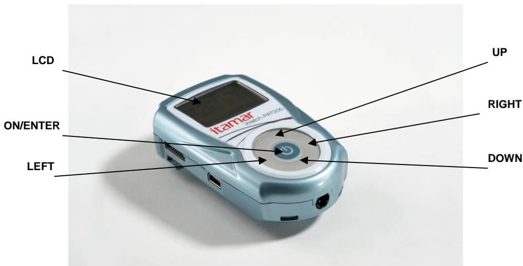
**Figure 3 – The Buttons and Display**
