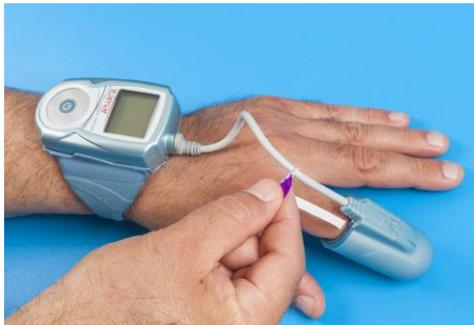
Figure 24 – Removing TOP Tab
