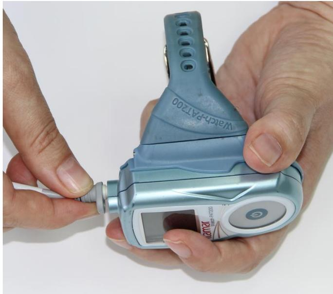
**Figure 18 – Replacing the uPAT Probe**
