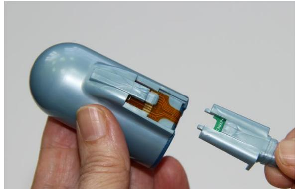
**Figure 8 – Probe Disconnected**
