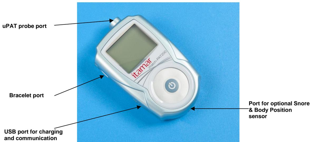
**Figure 4 – Service Ports and Peripherals**
