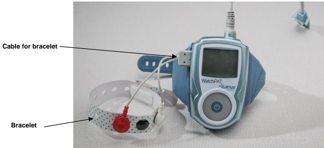
**Figure 10 – WatchPAT™ Device with Tamper-Proof Bracelet**
