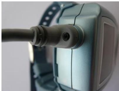
**Figure 17 – uPAT Probe Cable with Screw**
