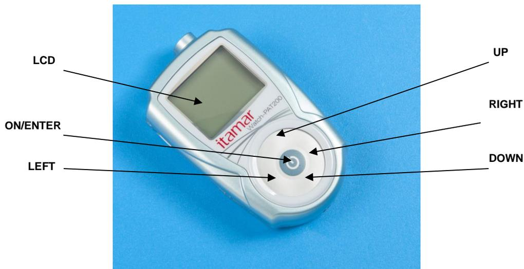
**Figure 3 – The Buttons and Display**
