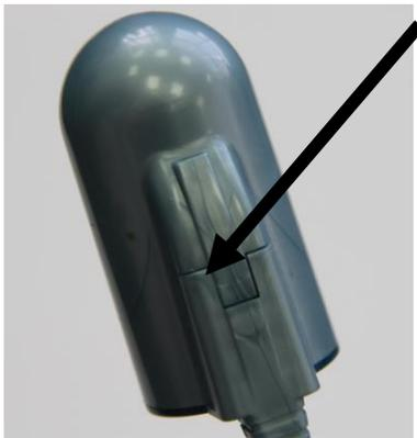
**Figure 6 – Disconnecting the Probe**
