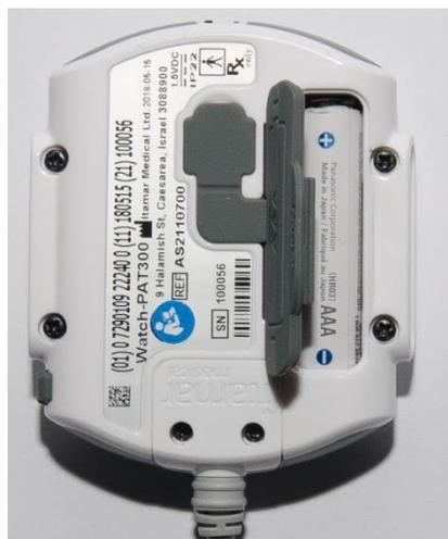
Figure 5 – Battery Compartment
