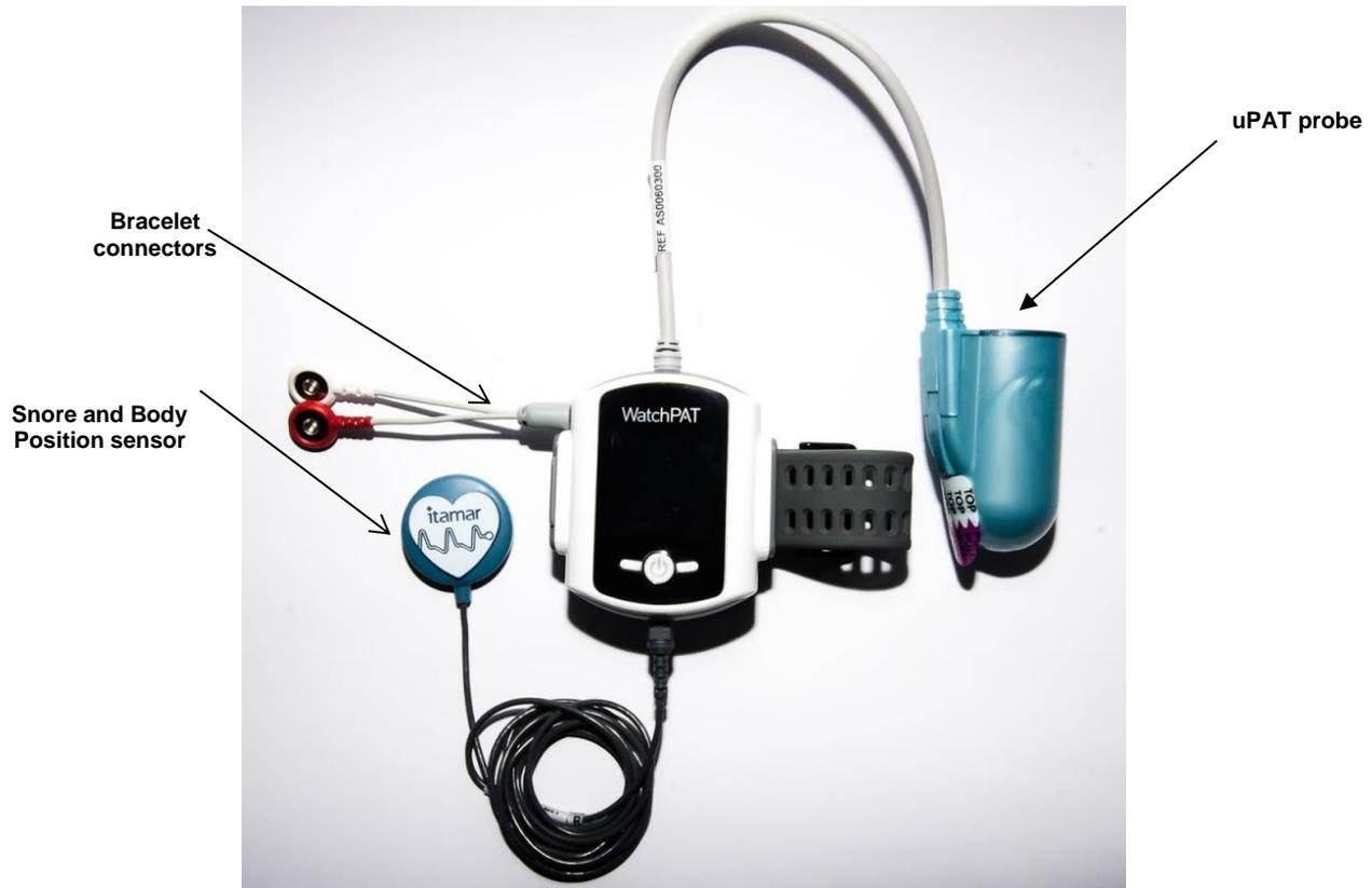
Figure 8 – WatchPAT™ Fully Prepared
