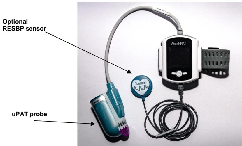
**Figure 2 – WatchPAT™ 300 Device with Sensors**
