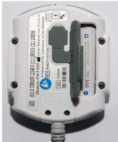
**Figure 5 – Battery Compartment**
