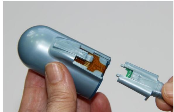
**Figure 7 – Probe Disconnected**
