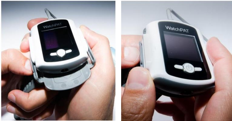
**Figure 20 – Seating device on wrist strap**
