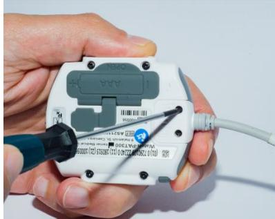
**Figure 16 – uPAT Probe Cable with Screw**
