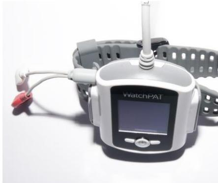
**Figure 11 – WatchPAT™ 300 Device with Cable for Bracelet**
