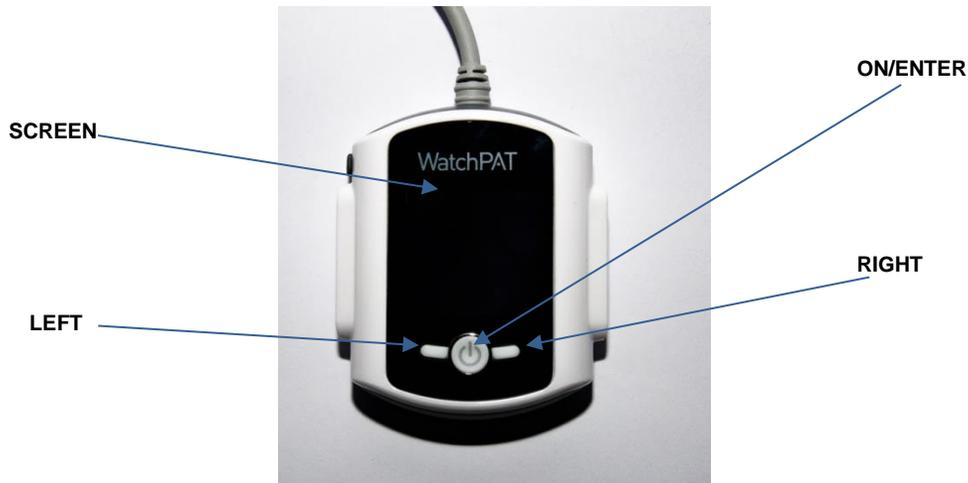
Figure 3 – The Buttons and Display
