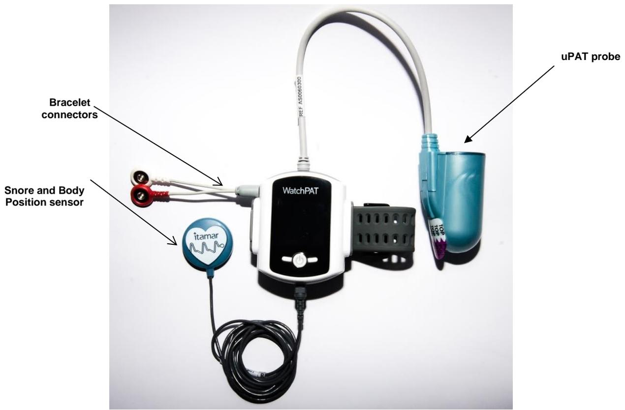
**Figure 8 – WatchPAT™ 300 Fully Prepared**
