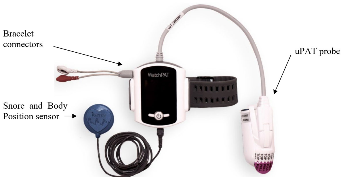
Figure 8 – WatchPAT™ 300 Fully Prepared
