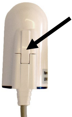
Figure 6 – Disconnecting the Probe
