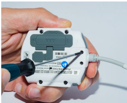
Figure 16 – uPAT Probe Cable with Screw
