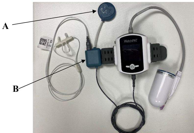
A – RESBP Sensor B – Interface (NAF-IM) to connect Thermal Airflow sensor
