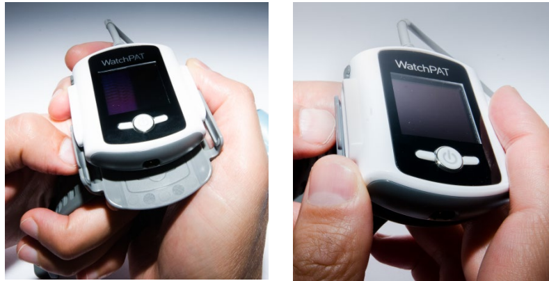
Figure 20 – Seating device on wrist strap
