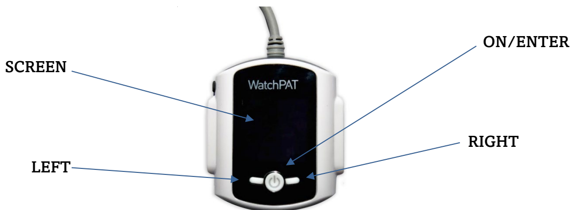
Figure 3 – The Buttons and Display
