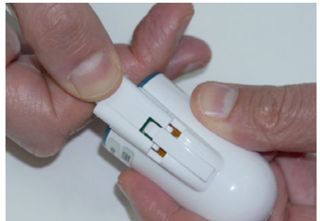
Figure 25 – New Finger probe connection
